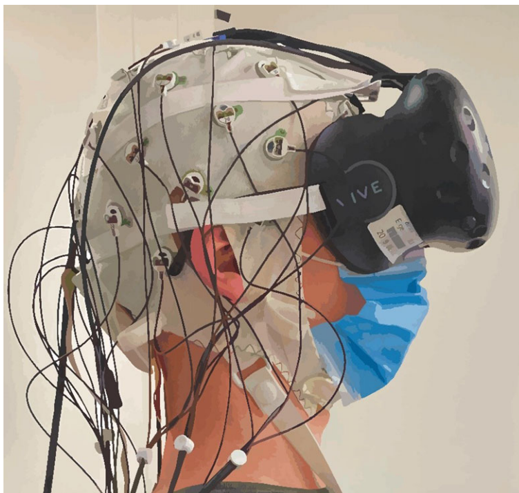
Figure 3. Set-up of the EEG recording and VR system on the participant. The electrode cap was fitted first before the VR system was mounted on the participant's head. The straps holding the VR system in place were carefully placed in-between the electrodes.
